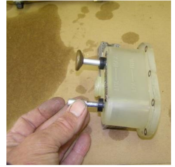
20. Mounting the dummy plungers. The copper disk presses the tube against the rubber seals
