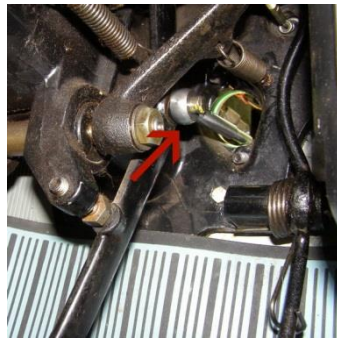
22. Important. Replace the pushrod at the brake pedal, it is longer than the original one!
