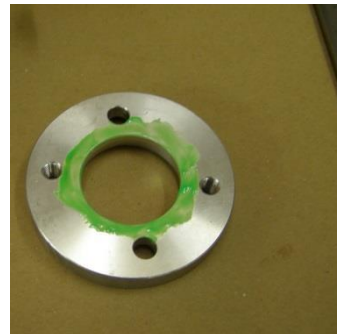
11. Thin coating of liquid gasket on the spacer.
