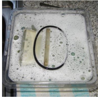
18. remove plungers and rinse container and sealing ring in warm soap solution
