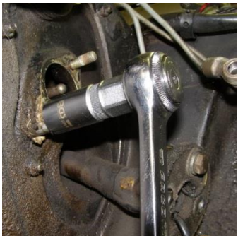
9. Remove the original studs with a suitable tool
