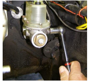
4. Removing the banjo bolts.
