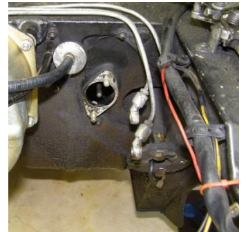
8. Old master brake cylinder removed.
