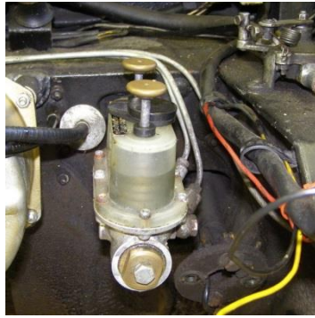
2. The old master brake cylinder.
