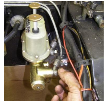
24. Fit the banjos but do not tighten yet. Fill some brake fluid in the reservoir and let it leak through. This facilitates later bleeding of the system. Use a suitable container to catch the spills. Then tighten up.
