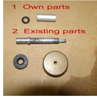
19. Modifying the old plungers for original looks. Aluminum pipe outer diam 8mm, length approx. 21 mm. Standard R03 O- ring
