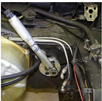
13. Torquing to 25 Nm should do (6mm bolt diameter)
